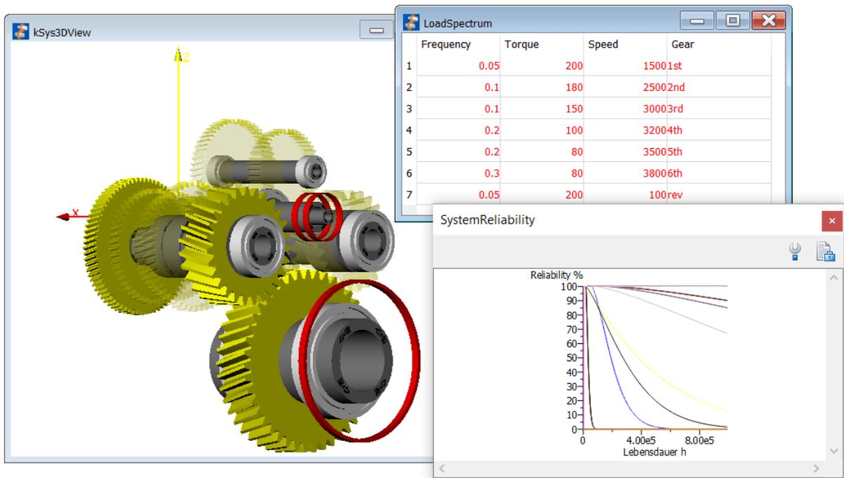
Figure 7 Modern dual clutch gear unit with a load spectrum (6 forward gears and one reverse gear)
