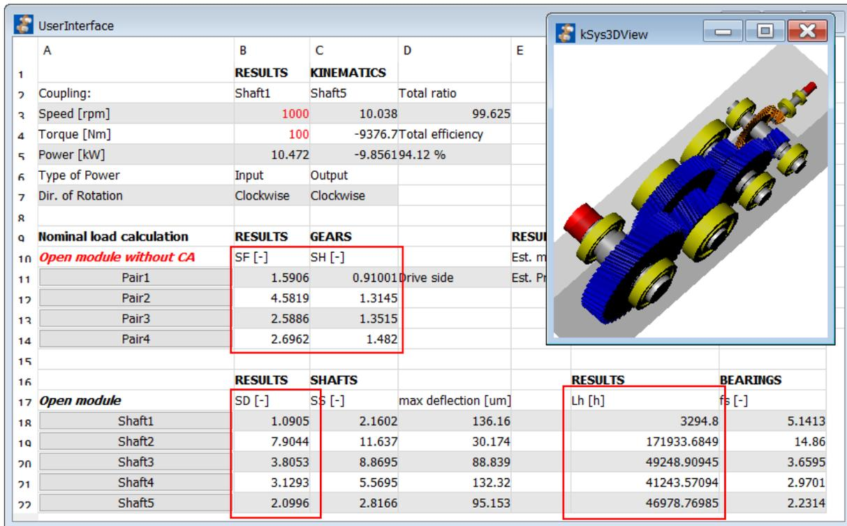
Figure 1 Overview of the results of a 4-stage bevel helical gear unit (SF: bending safety; SH flank safety; SD: safety of the most critical shaft cross section; Lh: bearing service life)
