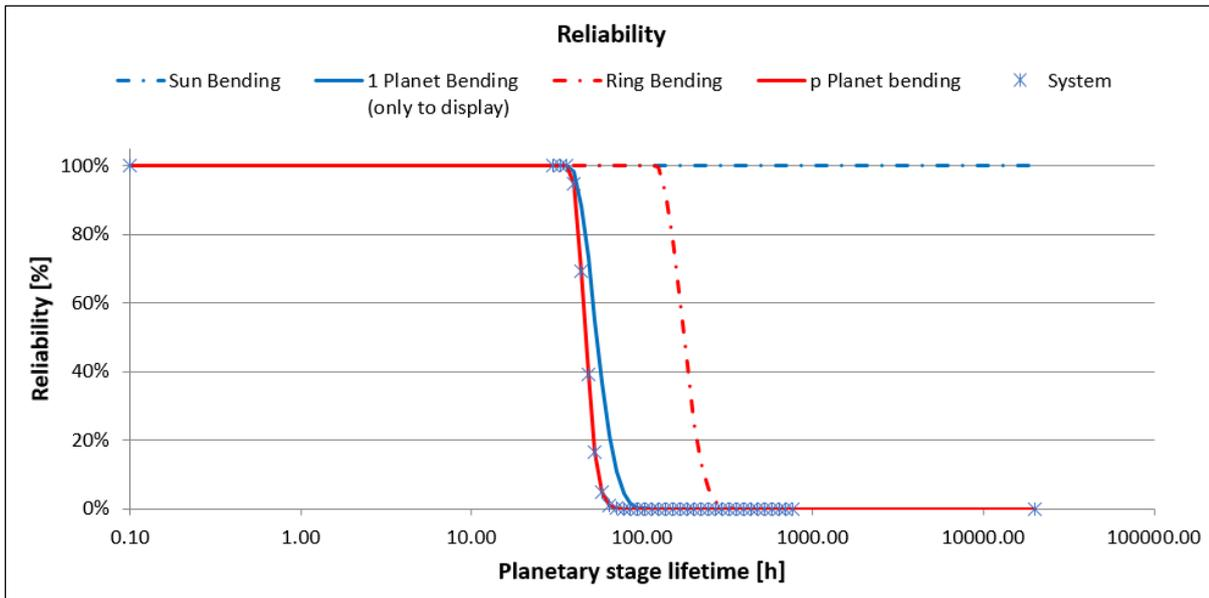
Figure 5 Reliability diagram for a planetary stage with 3 planets: the 3 serially cumulated planets are critical. The system reliability is virtually identical to the reliability of these 3 planets, because the ring and the sun have a significantly higher degree of reliability.
