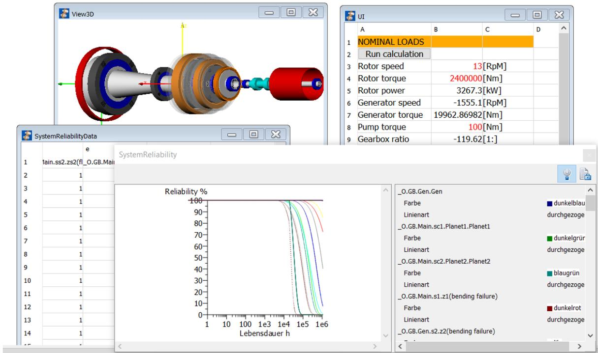
Figure 8 Wind power gear unit with it's reliability
