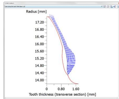
Wear is displayed either in 2D or in 3D and can provide a clear evaluation of the various modifications involved, for example, the effect of tip relief on the wear behavior.
